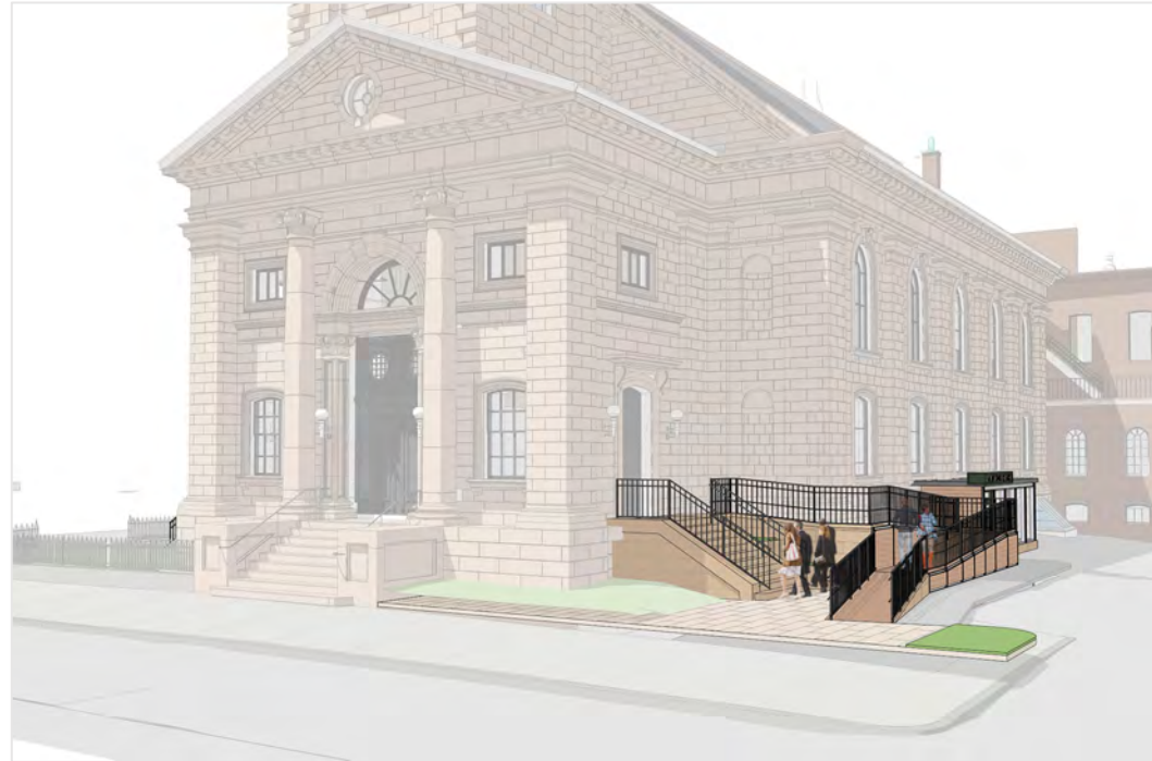
Stair and ramp intervention on north façade extends to Arlington Street where accessible parking and van drop-off make this ramp location convenient.
